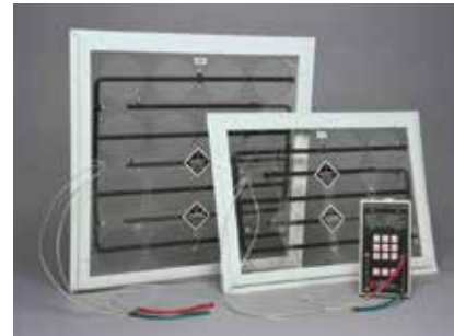
The TrueFlow® Air Handler Flow Meter, shown with DG-700, is used to measure the total amount of air moving through an air handler.
