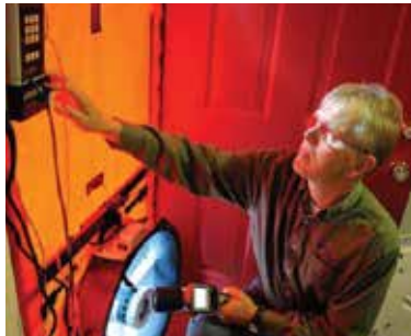
The Minneapolis Blower Door™ airtightness testing system.
