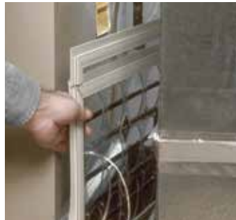
TrueFlow® Plate #14 with 2x20 spacer at filter slot between the return and the air handler.
